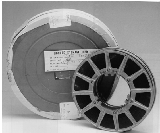
Figure 6 - Shown above is the actual spool of magnetic tape removed from the DSE used during Apollo 15. The 1" wide Mylar tape is shown contained on the original 8" diameter metal. This particular item sold to a private collector for nearly $3,000 during a Superior Galleries Space Memorabilia Auction held in May of 2000.
