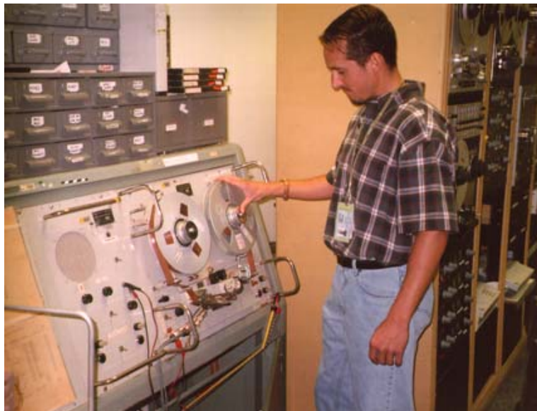
Figure 9 - Top photo shows copies of the original mission control audio tapes as they are stored in the Public Affairs vault at NASA's Johnson Space Center in Houston, Texas. Bottom photo shows the last remaining operational 30-track Soundscriber tape recorder as originally used in Mission Control. NASA JSC audio engineer Greg Wiseman is shown at work dubbing a tape to the newer recording equipment seen in the background. Photos courtesy of the author.
