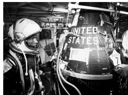
The three white squares on Faith 7 (arrow), covered over by clear plastic and tape during the pad tests. Credit: NASA
